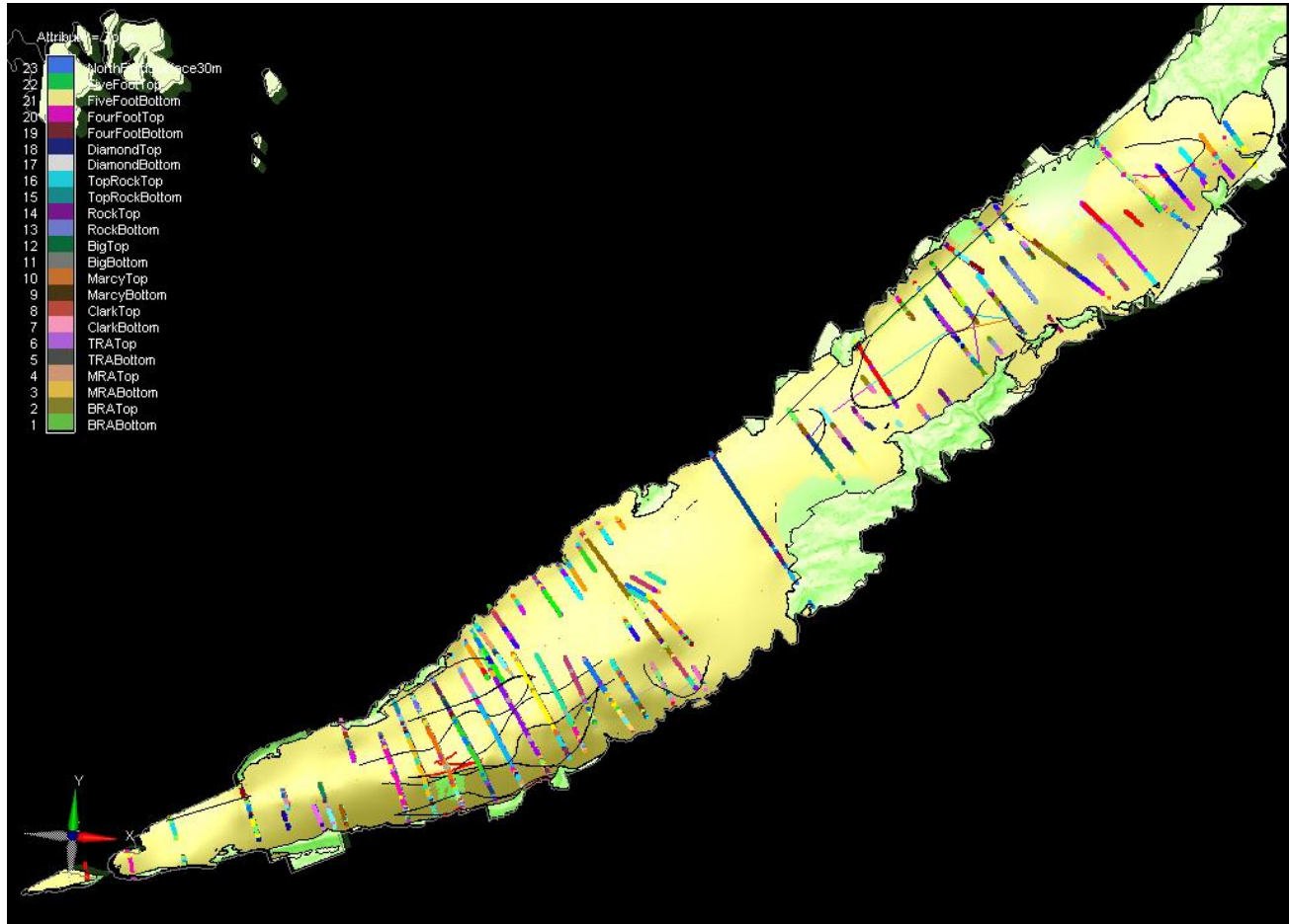
Figure 47: Resulting 3D model of combined Wyoming and Lower Lackawanna Valleys scattered cross section data. 11 individual coal veins are represented with true 3D grids.
