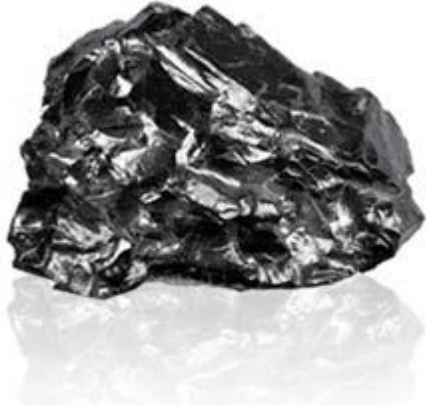
Figure 3: Anthracite coal is generically a called “hard coal” mineral because it is of higher rank on the carbon scale (i.e. harder) than the coal beds of the Bituminous Coal Region of western Pennsylvania, its high luster, high carbon content, typically between 92-98%, and relatively few impurities (Stefanenko, 1983).
